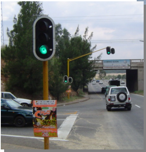
The efficient use of backboards to ensure contrast against a variable background
